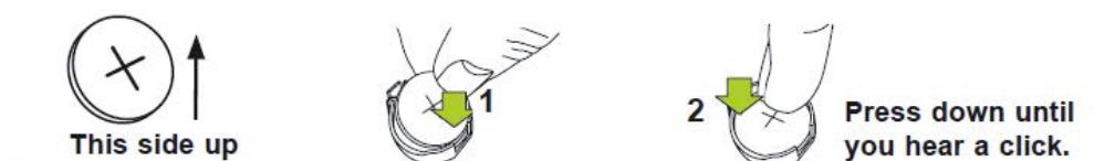
Figure 19. Install the battery
